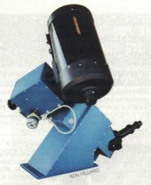
third diagonal is mounted on the tilt axis and rotates at half the tilt's rate to keep the image centered in the eyepiece. The eyepiece tube can also be extended or retracted by about seven inches. Since the second achromatic lens is mounted inside the eyepiece tube and the light rays have been made parallel by the first lens, the eyepiece's focus remains unaffected by this adjustment.
