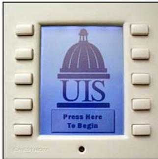
ⓘ If the Crestron LCD display is blank, touch the panel or press any pushbutton to activate the Crestron system.
