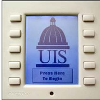
**ⓘ** If the Crestron LCD display is blank, touch the panel or press any pressbutton to activate the Crestron system.
