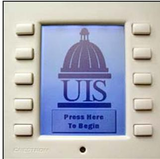
**i** If the Crestron LCD display is blank, touch the panel or press any pushbutton to activate the Crestron system.
